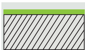
2. Indicator layer Apply RILUMINATI 815 evenly and thinly
