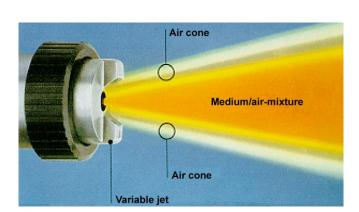
Notice: For usage a pressure of 1,8 bar is necessary!
