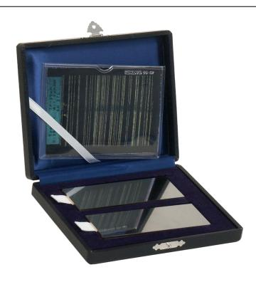
The reference test block JIS Z 2343 consists of two rectangular panels with transverse grooves and a NiCr-Coating. The thickness of the coating, and thus also the depth of the grooves, will vary between 10 to 50 μm, depending on the application.
