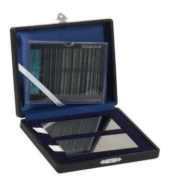
The Reference test block 1 acc. to EN ISO 3452-3 serves for the control of the sensitivity to indiation of liquid penetrants.
